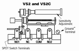
\*The internal ground connection is only available on the VS2 by threading the nut supplied in the hardware kit onto the base mounting bolt,
